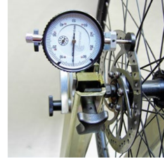
Brake disc measuring device only Comfort model
