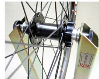
Support for universal quick release axles up to D 28mm
